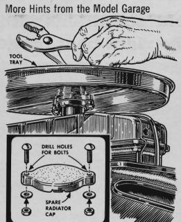
A tip-proof tool tray can be made by bolting a large pie tin or serving tray to the top of a spare radiator cap. Mounted on the radiator's filler neck in place of the regular cap, the tray is right at hand as you work in the engine compartment.
