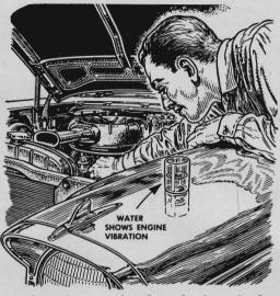
A glass of water placed on the front fender will guide you when adjusting the carburetor. Turn the idling screws in or out until the water is least agitated. At this point, jets will be set for smoothest idle.
