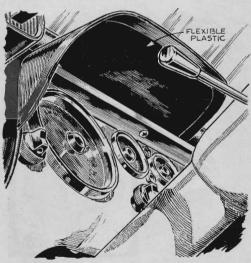
A plastic "eyebrow" can kill windshield reflections from a lighted instrument panel. Cut it from flexible opaque sheet, loosen the molding enough to slip the edge under, then retighten. If dash lacks molding, driff holes for sheet-metal screws.
