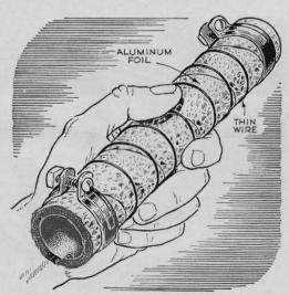
Radiator and heater hoses are too often located near oil dipstick tubes and valve covers, where they get coated with oil and start to deteriorate. To prevent this, give such hoses a jacket of foil, held in place with a wrapping of light wire.
