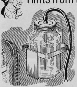
Windshield washer reservoirs need distilled water in hard-water areas—but it's not always easy to come by. For a substitute, collect water from melting ice when you defrost your refrigerator or from the plastic drain pan of an electric dehumidifier.
