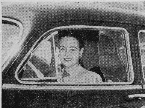
**Eliminates Drafts.** Even though the front window of a car is wide open, a plastic device made by the NuWorld Products Company, Huntington Beach, Calif., deflects the wind outward, protecting rear-seat passengers from drafts. Installed inside the window by three clips, it does not interfere with normal window operation.
