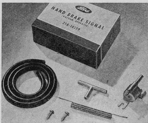
**Warns That Brake Is On.** A new Ford accessory gives audible warning if you start out without releasing the hand brake. Vacuum operated, it consists of a whistle, a hose and T-shaped unit for connecting to the wiper vacuum line, and a spring to hold the whistle open while the brake is set. It blows only when the engine is running.
