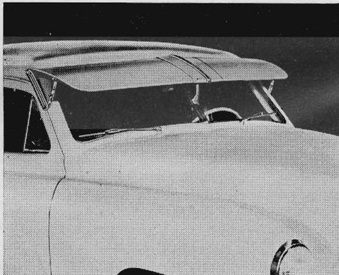
**SHADE CUTS SKY GLARE.** A sheet-aluminum shade with stainless-steel and chrome-plated brass fittings affords drivers protection against overhead glare. It is made by the Fulton Company, of Milwaukee, in sizes to fit most popular and de luxe models of 1942, 1946, and 1947 cars and many others of older make.
