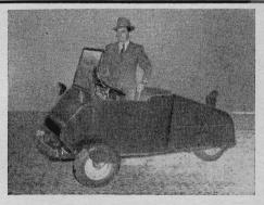
fore coming to the United States, this one had a single-beam frame, a radiator on each side of the 4-cylinder engine, and four speeds forward. It could attain a speed of 85 m.p.h. The streamlined front fenders were shaped to the wheels and moved with them when the car was steered.
