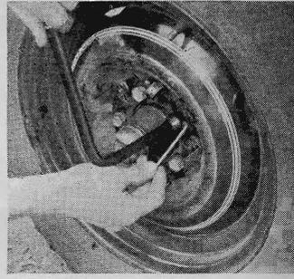
**TIRE THEFT** is made extremely difficult if you make use of the simple procedure outlined in the photos and drawings above. In principle, the method consists of rounding one tire-retaining nut or bolt so that it cannot be turned by a lug wrench without a special key. The idea is adaptable either to the nuts or the bolts variously used with pressed-steel wheels.
