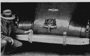
WOODEN BUMPERS made of laminated maple bonded with a resin adhesive, like the one at the left, have been subjected to tests that indicate they will withstand an even greater shock than comparable steel bumpers. As an additional advantage, it is claimed for the wooden bumpers that they can be polished very quickly if scratched. Even chunks chipped out of them can be replaced and the scars hidden beneath a new finish. The weight of the laminated type is slightly less than that of steel bumpers.
