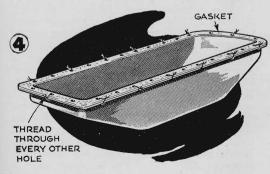
4 GASKETS CAN BE HELD in place by thread when an oil pan (or any other large part using a gasket) is being reassembled. It is often difficult to insert the bolts through the proper holes even when heavy grease or shellac is used as a binder for the gasket. If ordinary sewing thread is looped through alternate holes, the pan can be bolted on easily. Once the bolts are drawn up tightly, the fine thread will not interfere with a perfect seal.—J. K.
