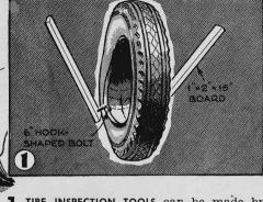
TIRE INSPECTION TOOLS can be made by inserting two 6" long screw hooks a short distance from the ends of two boards. If these are hooked over the beads of a casing and the ends of the boards are then pulled away from the tire, it is easy to look for breaks, other injuries, or nails. The tools cost little to make and may be conveniently carried in the car.—A. R.
