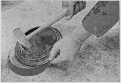
A HUB-CAP DOLLY and a plastic hammer are the answer to the problem of straightening out dented hub caps. Six inches in diameter and weighing seven pounds, the iron dolly has two concave surfaces—a deep one for the smaller caps and a shallow one on the other side for the larger.
