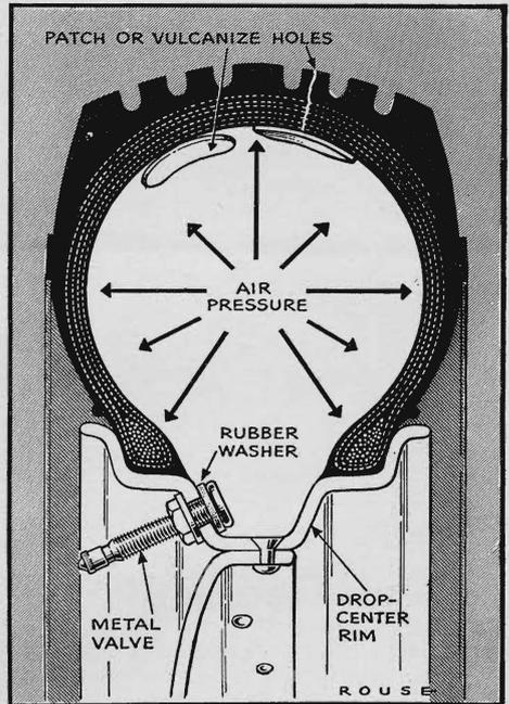
IF YOU have four tires but are short an inner tube, you can drive without it, says J. B. McGay, a Tulsa, Okla., manufacturer, who has worked out a method of mounting ordinary casings without tubes so that they can be inflated and run at normal speeds. About 700 tires so mounted are in operation in Tulsa alone, some of them having run as much as 12,000 miles in three months. The casings, it is reported, lose no more air than do tires with tubes.
