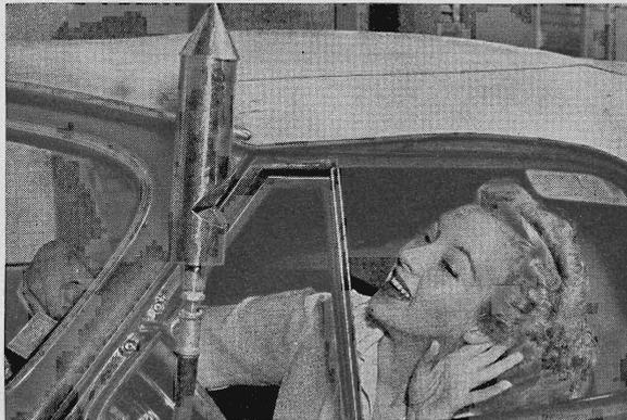
**A SPEED-LIMITATION HORN** for gas-and-rubber-saving drivers, toots its warning when the speedometer needle makes contact with a button set at the 35-mile mark on the dial. Contact opens a valve in the exhaust, which in turn blows the horn.
