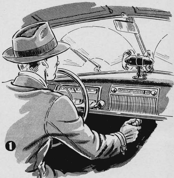
**1 DEFROSTER FANS**, which frequently are furnished new with plain on-off-type switches, can be made more flexible by replacing the original switch with a rheostat type such as most heater blowers have. The rheostat switch, available at most automobile-accessory stores, costs but a few cents and attaches easily under the dash.—P.V.
