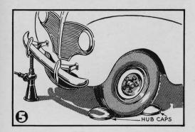
5 WHEEL BLOCKS to prevent the car from rolling backward or forward off its jack while a tire is being changed are handy to most motorists without their realizing it. Such blocks are afforded by the removable hub caps which the majority of cars have. Use one from the wheel that is to be changed and which must be removed anyway. Take the other from the opposite wheel. One before and one behind this wheel will prevent the car from rolling in either direction.—L.R.
