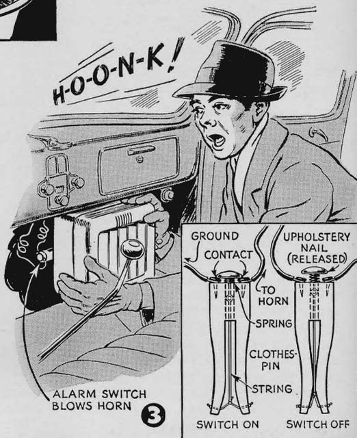
**3** **A BURGLAR-ALARM SWITCH** attached to your horn and placed behind the heater blows the horn if the heater is removed. Cut and drill a clothespin as shown. The center string is tied to a hook bent in the point of the upholstery nail whose head forms the switch contact when the removal of the heater allows the feet of the clothespin to spread.—P.M.
