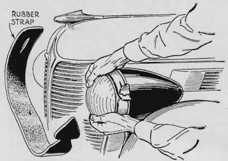
LOOSENING and removal of lens rims from headlights on cars several years old is simplified considerably if a tongue strap cut from an old inner tube is employed in the manner shown in the sketch above. The strap is stretched around the lens rim and the tongue slipped through the slit to hold it firm while the lens is being removed from the lamp.—G. E. H.
