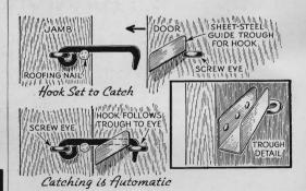
MY GARAGE has a sliding door which hooks on the inside. I found it a nuisance always to have to lock the hook and screw eye from the inside and then leave by the side door. The simple arrangement shown above solved my problem. A sheet-metal track screwed to the door guides the hook as the door shuts, dropping it into the screw eye. A large-head nail holds the hook so that it enters the track properly .- F. H.
