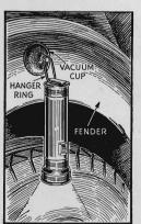
car will increase the light's usefulness. When changing a tire at night, for example, you can throw the light right onto the work by attaching the vacuum cup to the fender above the wheel. In the same way, it may be fastened to illuminate the motor or the trunk compartment, or any other spot where light is needed .- E. F.
