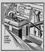
ON LATE-MODEL automobiles that have their batteries underneath the hood, any possible damage to wiring and metal parts can be prevented by stretching a section of inner tube two inches wide around the top edge of the battery. This keeps acid from spreading if the battery is overfilled .- E. J. C.
