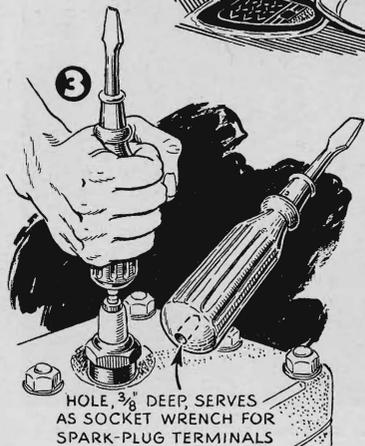
HOLE,  $\frac{3}{8}$ " DEEP, SERVES AS SOCKET WRENCH FOR SPARK-PLUG TERMINALS
