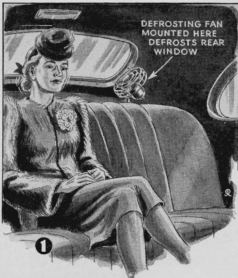
**1 AS A SAFETY FACTOR** for winter driving, as well as a convenience, an electric defroster fan mounted on the deck space behind the rear seat of a car and aimed at the rear window is as effective as one used on the windshield. It keeps fog and frost from forming on the inside, and melts snow and sleet that gathers on the outside while parked or driving. It may be easily wired from the ammeter and ground through a dashboard switch.—W. P. H.
