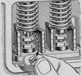
Removing Valve Keys. If you lack the proper lifter, here's how you can remove valve keys from an L-head. Hand-crank the engine until the valve opens and slip two flat files (you need a nonslip surface) on edge under the spring. Crank engine to lower valve, and you can pull out the keys. It works in replacing them, too.
