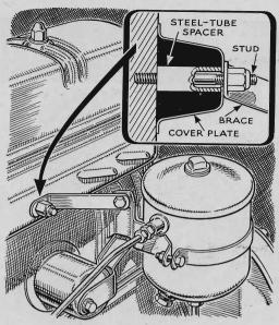
**Spacer Anchors Oil Filter.** On some latemodel Buicks, the oil-filter bracket is fastened to a cover-plate stud. A metal spacer slipped on the stud behind the cover provides a solid base against which to tighten the nut. This makes it less likely to rattle.
