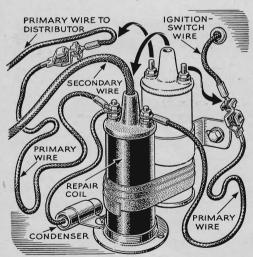
**Save a Towing Bill.** A bad coil or condenser accounts for many breakdowns. One veteran mechanic takes this spare coil and condenser unit on road calls, and he reports it often enables him to drive the car away. Carried in the car, such a unit may save any motorist a towing bill. Ground the condenser shell.
