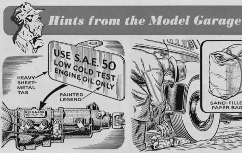
Tag Shows Proper Lubricant. In some new cars, a heavy motor oil is specified for the transmission instead of grease. To prevent careless errors, paint the oil recommendation on a metal tag and attach it near the transmission filler plug.
