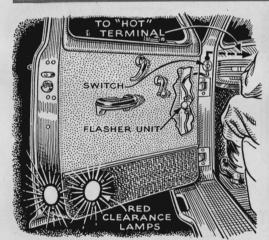
Door Lights Flash Warning. Before getting out the driver's door in traffic, it's always a good idea to look both ways. John W. Bell, of Des Moines, Iowa, has provided additional safety with this warning system. When the door is opened, a normally-off push switch in the door jamb shoots current to the flasher unit. An auxiliary switch on the dash cuts off the system if you want to keep the door open.
