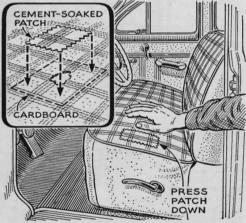
Patching Seat Covers. You can repair a worn area or tear in fiber seat covers by cementing on a patch. Cut the patch from a hidden part of the cover, using pinking shears if available. Put cardboard between the worn area and the upholstery to protect the latter, saturate the patch with clear model-airplane cement, wait until it is tacky, and press firmly in place. Let the patch dry overnight.
