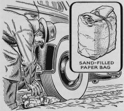
Sand "Bombs" Overcome Ice. If you frequently must drive on ice, keep sand in your luggage compartment, packaged in paper bags tied with string. Carry the bags in a cardboard box. Then, when stuck, drop bags under the rear wheels.
