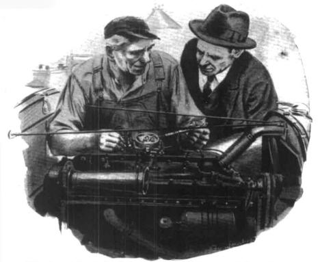
With a loop of wire Gus hooked a spring balance to the spring in the breaker arm. "Look closely," he said, "and you'll see that the balance reads about eighteen ounces."
