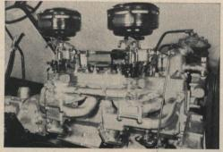
Twin advantages of high-power output and low-operating cost are claimed as a result of several twin features in the engine above, designed for Dodge's new Y and YA model four-ton trucks. The engine, developing 330 pound-feet torque, has twin carburetors, twin manifolds, and a twin exhaust system. The new six-cylinder power plant delivers 154 hp., has a 6.5 to 1 compression ratio, and a displacement of 377 cubic inches.
