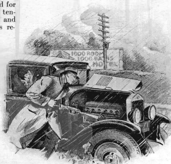
Fire extinguisher fluid dries out rain-soaked ignition system and helps start the motor.
