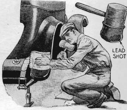
Fig. 1—Straightening bent fender with a sand bag and mallet faced with lead shot
