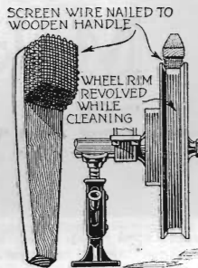
Fig. 3—A quick way to clean a rim with a screen wire brush
