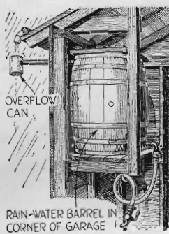
Fig. 3. How to install a barrel in garage to supply rainwater for the radiator
