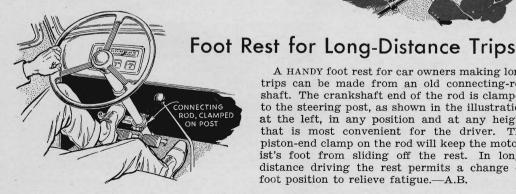
A HANDY foot rest for car owners making long trips can be made from an old connecting-rod shaft. The crankshaft end of the rod is clamped to the steering post, as shown in the illustration at the left, in any position and at any height that is most convenient for the driver. The piston-end clamp on the rod will keep the motorist's foot from sliding off the rest. In longdistance driving the rest permits a change of foot position to relieve fatigue.—A.B.
