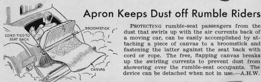
PROTECTING rumble-seat passengers from the dust that swirls up with the air currents back of a moving car, can be easily accomplished by attaching a piece of canvas to a broomstick and fastening the latter against the seat back with cord or rope. The free, flapping canvas breaks up the swirling currents to prevent dust from showering over the rumble-seat occupants. The device can be detached when not in use.-A.H.W.
