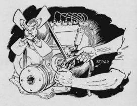
USE of a leather strap helps when installing a new fan belt on a car. Place the fan belt over the fan and crankshaft pulleys, and loop the strap around the fan belt as in the drawing above. Pulling the looped strap makes it an easy matter to stretch the new belt so that it easily slips over the generator pulley.-N.V.
