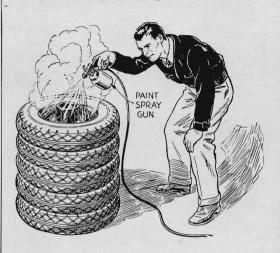
WHEN painting wire wheels, you can save yourself time and trouble by piling the wheels one on top of the other and spraying down through the whole batch. The rims form an inclosure that prevents the spray from spreading, and each wheel gets well covered. Excess paint can be removed with a gasoline-dampened rag.—A.C.M.
