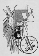
I've often struggled to retrieve a bolt or nut that dropped down beside the motor of my car, but recently I stumbled on an easy and effective method. Merely split the end of a twig and use it as a long - handled clothespin to grab and lift the elusive part, as shown in the drawing at the left.-L. M.
