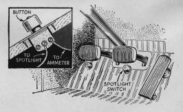
A HEADLIGHT dimmer switch is a convenience for turning a car spotlight on or off. When driving at night, the spotlight switch, placed on the floor between the clutch and brake, makes it unnecessary for the motorist to take his hand off the wheel to cut out the spotlight as another car approaches. How the auxiliary switch is installed is pictured in the drawings above.—R. E. S.
