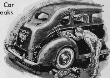
An irregular roller reproduces the ef-fect of a rough road
