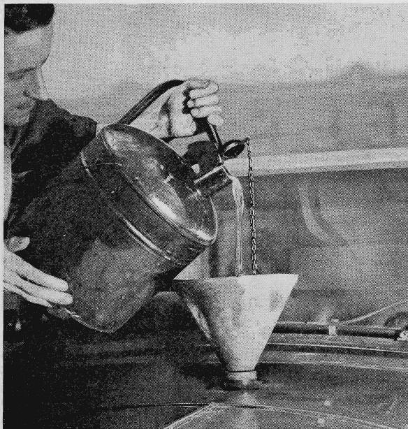
Chain fastened to the spout carries off static electricity
