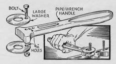
Washers mounted on a pipe-wrench handle enable it to grip cylinder-head studs
