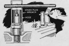
BECAUSE socket-type spark-plug wrenches sometimes break the porcelain around the plug as they are slipped on or off, I cut a short piece of rubber hose to fit snugly inside the wrench. Forced into the tool so that it clears the lower shank that grips the base of the plug, the rubber hose within the hollow tool acts as a cushion to protect the plug's porcelain insulator from accidental breakage.—A. M. C.
