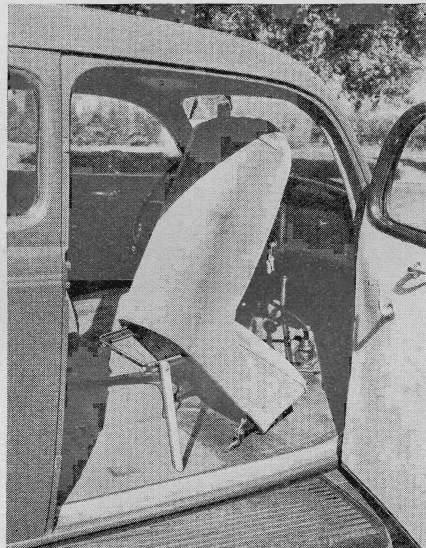
How the prop holds the front seat up to allow easy access to the rear of a two-door sedan
