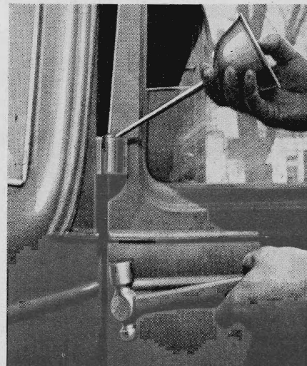
Tapping the bottom of the hinge pin with a hammer forces the oil to all parts of the pin
