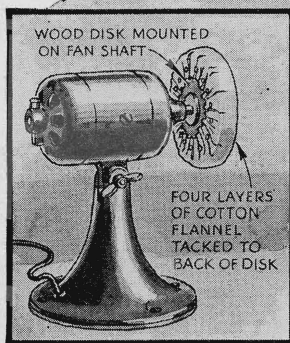
A padded disk, fitted to the shaft of an electric-fan motor, makes car polishing easy
