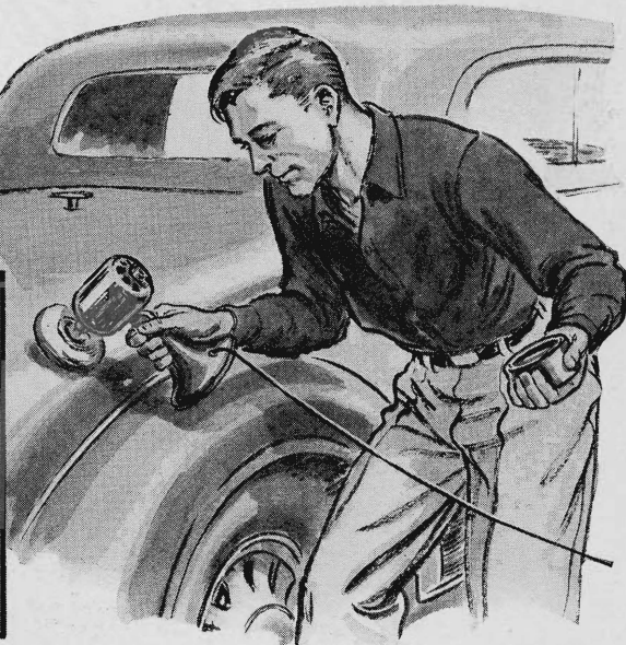
A padded disk, fitted to the shaft of an electric-fan motor, makes car polishing easy
