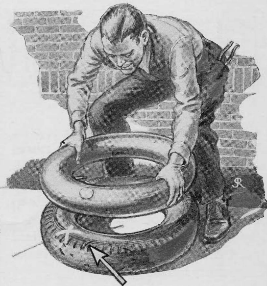
Chalk mark on tire casing helps to locate puncture
