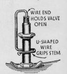
Drawing shows how to make wire device that depresses pin in valve stem and so releases air
