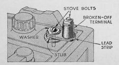
the terminals. It had broken off so close, that not even a slight projection remained to serve as a terminal for the clamp. After trying several ideas without success I made the temporary terminal shown in the sketch. From a small
