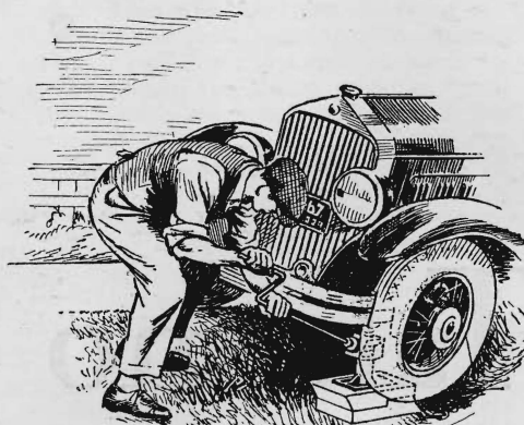
Fig. 1. Jacking up a car on uneven or rutted ground is easy if you have these blocks to put the jack on and chock the car. At right are shown the blocks ready to use if both wheels are to be jacked at one time.
