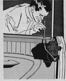
Window-button rods that drop down inside a car door can be retrieved with this simple tool: a conical spiral of tightly coiled copper wire, brazed or soldered onto a 6" length of 3/32" rod. The tight coils easily engage the threads of the button rod for lifting it.
