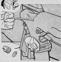
To free a stuck heat-control valve on a Dodge 318 V-8, you don't have to remove the exhaust manifold. Drill and tap a small hole just above the port and use an oilcan to inject a suitable solvent. Work the valve loose by moving the counterweight. Install pipe plug.
