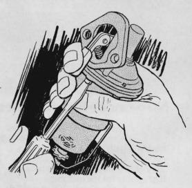
Frequent fuel-pump failure is usually caused by broken diaphragms. To make a diaphragm last longer, install it this way: Assemble the pump, leaving the screws loose. Operate the arm, and when the diaphragm is stretched fully, tighten the screws.
