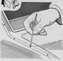
When moldings have been replaced, rust may develop around the molding fastener holes. Reason: Tightening the screws cuts through the paint. Put in a few extra minutes applying a drop of shellac or varnish to each of the screw holes to seal out the moisture.
