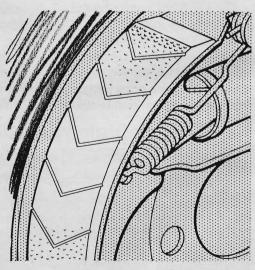
Squeaks from bonded brake linings can be eliminated by cutting V-shaped grooves in the linings, pointing in the direction opposite to the drum's rotation. This lets air carry dust to the outer edge of the shoe, where it can cause no vibration or squeal.
