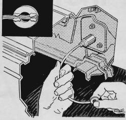
A stuck speedometer head can be fixed with a simple tool made up of a short length of old speedo cable with a flat washer welded or brazed to its free end. The keyed end is inserted in the instrument, and the cable twisted alternately to right and left.
