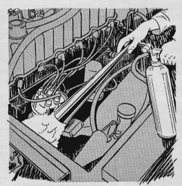
If you can't time your ignition because the distributor is stuck, all is not lost. You can free it with a CO2 fire extinguisher. Aim its nozzle below the distributor base and spray for about 10 seconds. This treatment will usually free the most stubborn unit.
