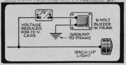
When backing up, you can alert children with this alarm: Add a six-volt buzzer to the car's electric system by mounting the unit inside the trunk and connecting it to the back-up circuit. The buzzer will sound when the car is in reverse.
