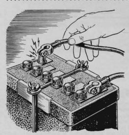
If the battery runs down frequently, you can suspect a small but constant current drain. This is checked by disconnecting one battery cable and touching it against the terminal. A tiny spark indicates that current is flowing. Check all wiring.
