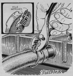
An old pair of slip-joint pliers makes a dandy tool for removing spring-type radiator-hose clamps. Notched as shown, it will hold a clamp without slipping. And you can work the pliers at various angles in those difficult or tight locations.
