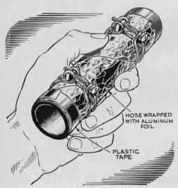
Radiator hoses—especially those at the bottom of the engine—deteriorate rapidly because of oil and dirt that accumulate on them. You can prolong their life by wrapping them with aluminum foil to keep them clean. Tape the ends of the foil.
