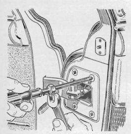
Extra leverage can be applied to a screwdriver with a nut welded on its shank. Press the screwdriver firmly into the screw slot and turn the nut with a wrench. The most stubborn screws can be removed this way without damaging them.
