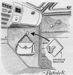
Handy hangers can be installed in your car at convenient locations without drilling holes. Use the plastic hooks with adhesive backing sold in dime stores. They come in various colors, and will stick to almost anything in the car.
