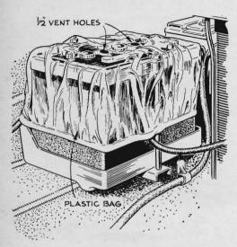
Protect the top of your battery from dirt and short-circuiting moisture, and cut down excessive evaporation of the electrolyte this way: Cover it with a plastic freezer bag. Cut two holes in the bag to vent off charging gases.
