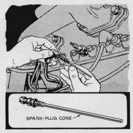
A spark tester, handy to use when spark terminals are sheathed in rubber, is easy to make this way: Break an old spark plug apart and save the core. The cap will snap easily into the wire terminal, leaving the core exposed for testing.
