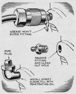
To clear a clogged grease channel, replace the fitting with a street elbow, fill the elbow with penetrating oil, and drive for a week. Put back the fitting and try your grease gun. Fresh grease should now force the old grease out.
