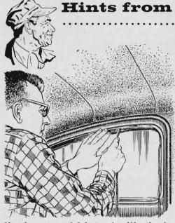
Here's a rope trick to simplify the installation of windows set in rubber molding. Place a heavy cord in the molding groove, press the window into position, and pull on the cord. The cord lifts the lip of the molding over the glass.
