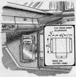
**Store road maps** in a small container screwed to the cowl paneling, and there'll be more room in the glove compartment. Cut the box from do-it-yourself aluminum sheet with household scissors. Bend it along the dotted lines.
