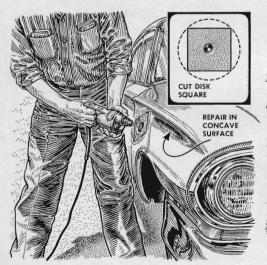
To avoid gouging concave surfaces with the edge of a portable disk sander, cut the disk into a square shape and mount it on the pad. Cutting action is lessened at the corners, yet the disk remains fully effective at the center.
